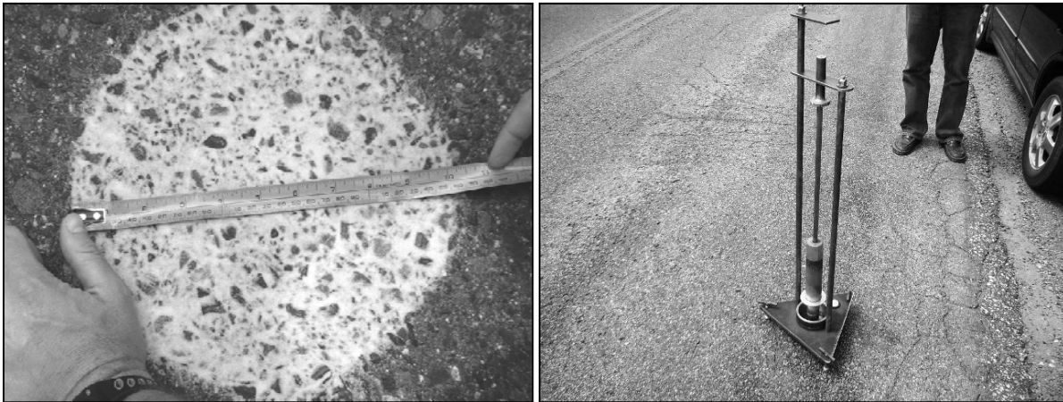
Figure 1. Sand Circle Test and Ball Penetrometer Used in Ontario
