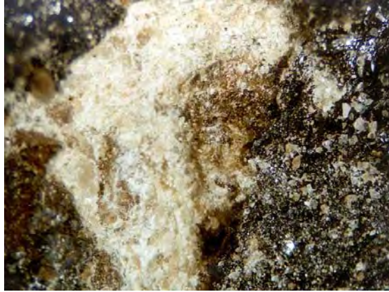
Figure 16. Microscope Photograph of Shattered Aggregate at the Bottom of the Rout in a Slab Cut from Highway 401 Westbound in Mississauga.
