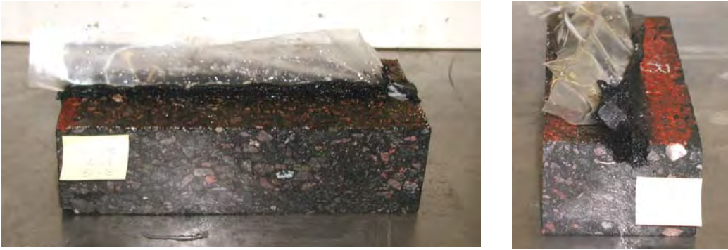
Figure 11. Sealant Bonded in Saw-Cut Reservoir After 8000 Cycles in the Asphalt Pavement Analyzer
