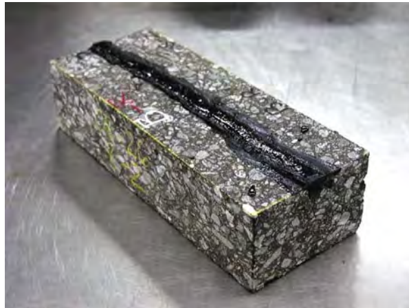
Figure 8. Sample with Routed Reservoir Filled with Crack Sealing
