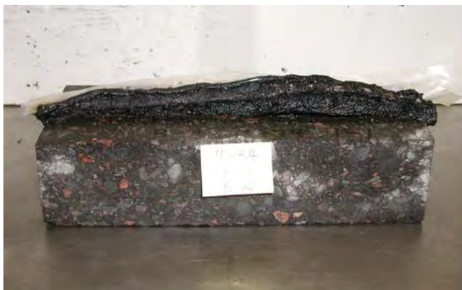
Figure 10. Sealant Debonded from Routed Reservoir after 2000 cycles in the Asphalt Pavement Analyzer
