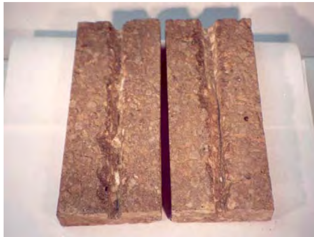
Figure 7. Samples taken from Runway 08-26 at Canadian Forces Base Goose Bay Ready for Crack Sealant Application
