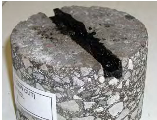
Figure 14. Cohesion Failure of Sealant in a Dry, Pull-out Test with a Saw-Cut Reservoir
