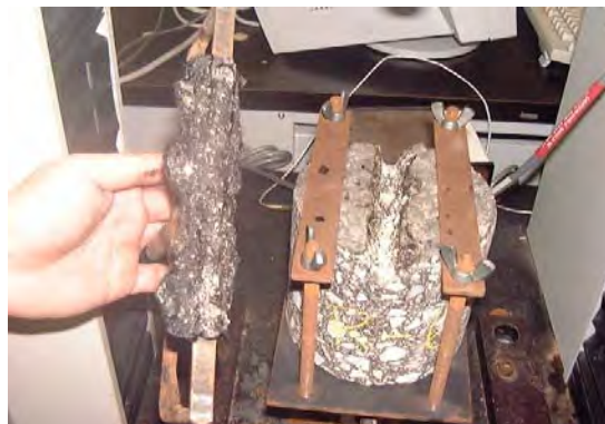
Figure 12. Adhesion Failure of Sealant in a Wet, Pull-out Test with a Routed Reservoir
