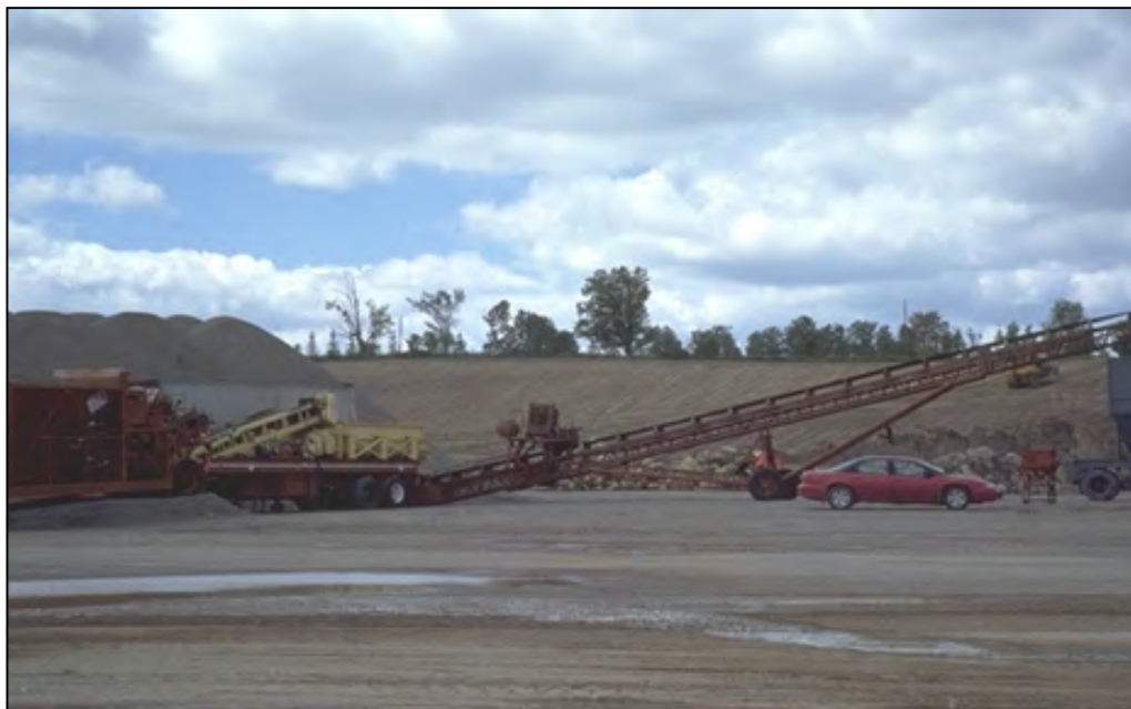
Figure 10 – Cold Mix Plant
