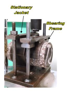
Figure 2-7 InstroTek© Testing Frame (Right) and Interlayer Shear Strenght (ISS) Apparatus (Left)
