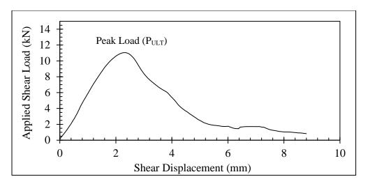
Figure 2-8 Typical Shear Load-Displacement Curve
