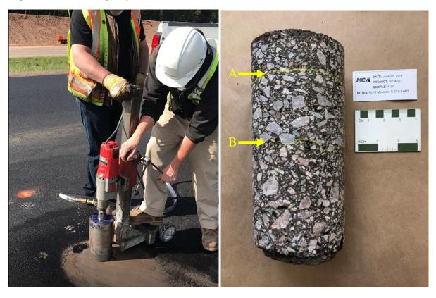
Figure 2-6 Coring Operation Using Pedestal and Support Column (Left), Interfaces
