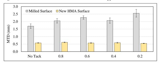
Figure 3-3 Mean Texture Depth (MTD) Measure Using Sand Patch Test
