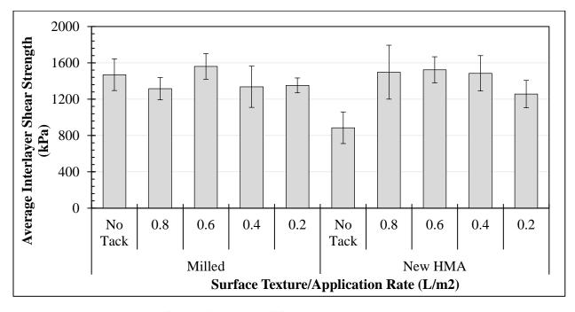
Figure 3-1 Interlayer Shear Strenght (ISS) Results
