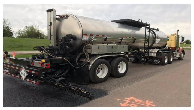
Figure 2-3 Etnyre Distributor Truck Used for the Study
