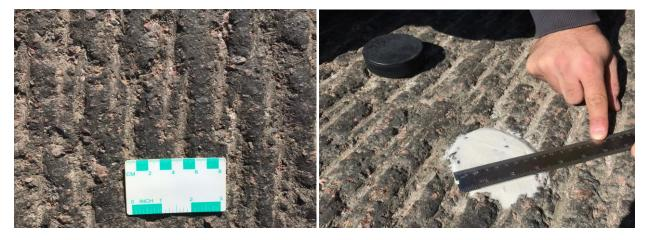
Figure 2-2 Milled Texture Prior to Application of Tack Coat (Left) and Measurement of Texture Depth Using the Sand Patch Test (Right)
