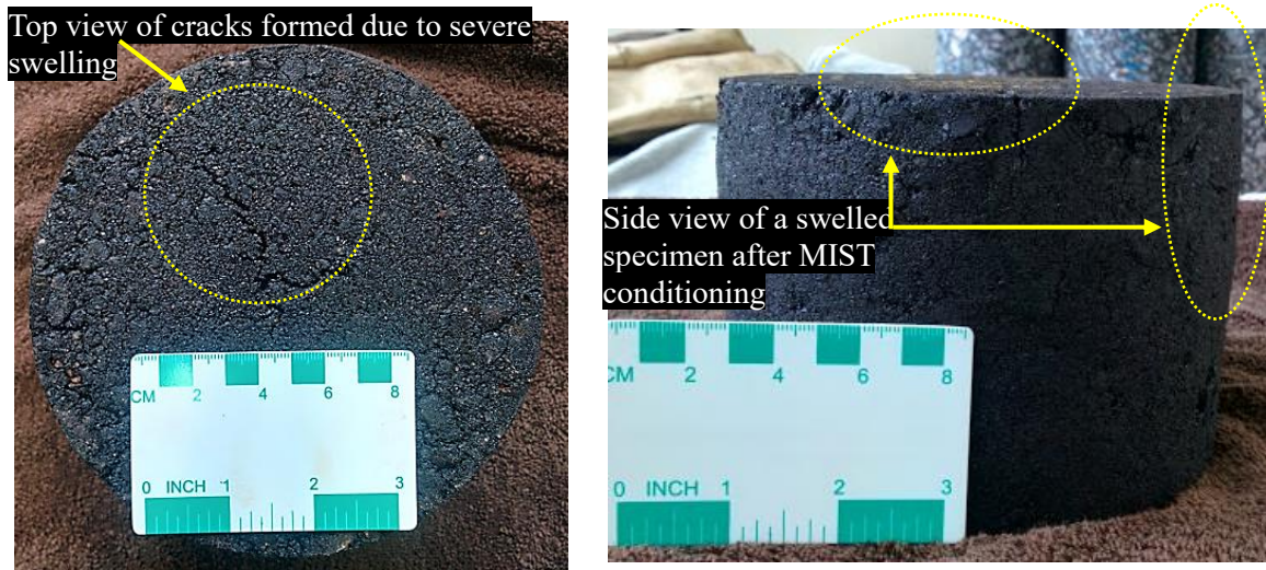
1 FIGURE 5 Severe Specimen Swelling Observed After MIST Conditioning
