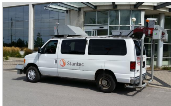
Figure 7. Vehicle Used to Collect Pavement Performance Data for York Region
