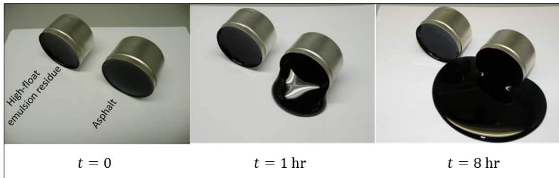
Figure 3. Flow behaviour of asphalt (right) and a high-float emulsion residue (left) formed from the same asphalt. The ambient temperature was 23°C.
