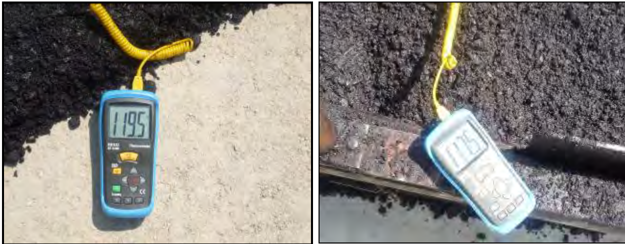
Figure 7. Rubber Asphalt Warm Mix Temperature in Paving
