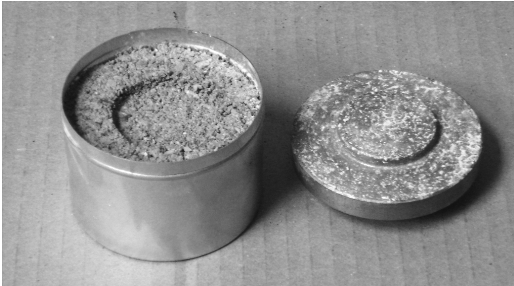
Figure 2. Compaction Plunger and Compacted Granular Specimen
